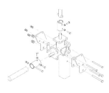
The roller Bevel Gearbox drive mechanism can be installed either side of unit. To change ends simply unbolt the 8mm mounting bolts (through square tube) to remove and turn the roller around
