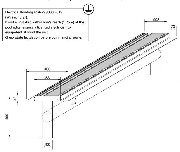
Length of DMR is to the outside of the unit. Prepare mounting for DMR to either sit on or be suspended under noting finished height of the unit should be finished paving/deck level
